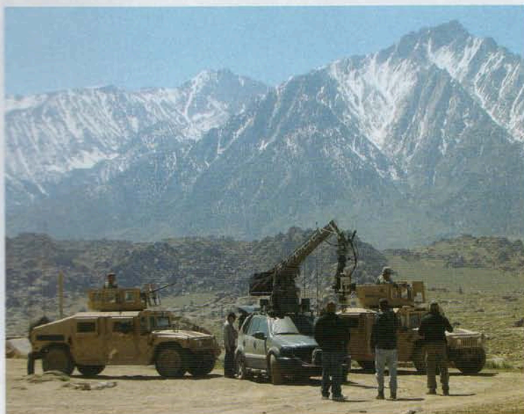
Left: The crew prepares to shoot on location in the Alabama Hills near Lone Pine, Calif. Below: The camera rig, which comprised eight Iconix HD-RH1 cameras, was mounted to a Flight Head III on a Z Crane attached to the top of a Mercedes ML55 SUV.
